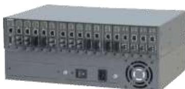
Fiber optic converter housing for max. 16 Fast and Gigabit Ethernet media converters of series 0961300D and 0961300M, 2HU, operating current: 90..264V AC, 60W, WxHxD 443x88x300mm, operating temperature -5°C..40°C, RH 5%..95% non-condensing, optional redundant power supply and / or management support.
