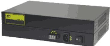
Power supply for devices with PoE and PoE Plus (high PoE) function, input 100..264V AC, output s. Selection box, cooling: Active fan, short-circuit proof, overload protection, EN60950, EN55022 class B, EN61000-3-2, EN61000-3-3, EN61000-6-2, dimensions 325x210x43mm 1HU, operating temperature 300W: -40°C up to +64°C (derating > 50°C), 1000W: -20°C up to +60°C (derating > 50°C), relative humidity 10% .. 95% non condensing.
