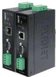
The device Server converts RS-232 or RS-422 / RS-485 COM ports according to Ethernet TCP/IP and vice versa. Serial: RS-232 at DB9, RS-422/RS485 at screw terminal max. 921600bps, Ethernet: 100Base-TX 10/100MBit/s Fast Ethernet RJ-45 port or 100Base-FX 100MBit/s fiber optic port, protection class IP30, operating temperature see selection box, dimensions WxDxH 135x97x32mm, input voltage 12..48V DC, consumption 10.1W, alarm contact for report of power failure, for fastening on 35mm DIN rail.
