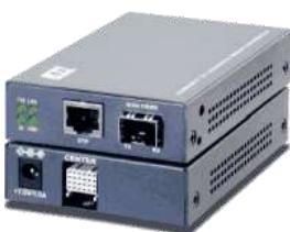
Gigabit Ethernet media converter with 1x 1000MBit/s 1000Base-T RJ-45 port and 1x SFP slot incl. 1000Base-X multimode / singlemode (monomode) or BiDi (WDM / SingleFiber) SFP module for LC connector. Direct media conversion, full wire speed, transparent, no packet length limitation. Operating temperature -5°C..55°C, RH 10..90% non condensing, dimensions 108x72.5x23mm. 19" mounting see product group 0961138 or 0961398. DIN rail see item 09611428 (selection box).
