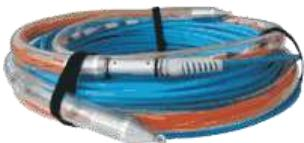
Rugged fiber optic loose tube outdoor cable with rodent protection, longitudinal- and radial water protection, A-DQ(ZN)B2Y, made-to-order termination multimode OM2, OM3, OM4 or singlemode (monomode) OS2 with connectors of your choice, optional on one side or on both sides with pulling- and protection element. DIN rail mountable by use of MPO/MTP connectors in combination with item group 12012062 possible. For indoor cable see item 018600004.
