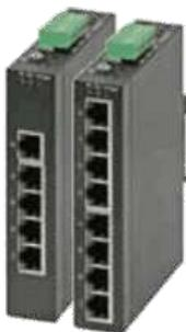
Fast Ethernet industrial switch, 5x or 8x 10/100Base-TX RJ-45 ports, auto MDI/MDI-X, IP30, rugged metal case dimensions 30x142x99mm (WxHxD), redundant power, polarity reverse protection, overload current protection (resetable fuse), operating voltage 12..48V DC / 24V AC, removable terminal block, extended temperature range -40..+75°C, wall mounting and 35mm DIN rail mountable (both included in scope of delivery).
