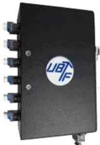
Fiber optic distributor box for mounting in a control cabinet on 35mm DIN rail, assembled with 12 fibers, 1x MTP/MPO to 6x LC duplex multimode or singlemode (monomode). Ready to use as plug-and-play installation s. Selection box.
