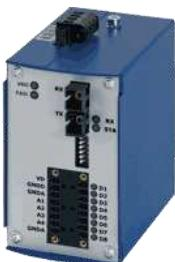
Fiber optic bridge for digital IO switching signals, 4x transmit 12V - 24V DC, 4x receive relay contact output. Optical fiber link wavelength 1310nm. Signal: Input (transmit) 12V - 24V DC / 5mA, output relay. Operating voltage 12V - 30V DC, consumption 5W, isolation 500V DC, operating temperature -40°C - +70°C, error relay output 25V DC 1A, housing stainless steel powder coated, dimensions HxWxD 115x61x113mm.
