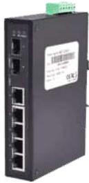
7-port Industrial Gigabit Ethernet switch with 5x 10/100/1000MBit/s 1000Base-T RJ-45 ports and 2x 1000Base-X/100Base-FX SFP slot for a multimode 1000Base-SX GbE, singlemode (monomode) 1000Base-LX GbE or a 100Base-TX Fast Ethernet SFP module. Jumbo frame support, reverse polarity protection, overload current protection, input voltage 12..48V DC, operating temperature: -40..75°C, rugged metal case IP30, dimensions WxDxH 30x99x142mm, FCC, CE.
