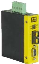
Fiber optic converter transmits RS-232 signals transparent via multimode or singlemode (monomode) optical fiber. D-Sub9 socket, DCE, transmits handshake (RTS, CTS, DTR, DSR), optical isolation between RS-232 and main circuitry, ESD-protection and overvoltage protection (RS232), relay signal contact for power failure, fanless metal case, dimensions WxDxH 28x82x95mm, mounting on 35mm DIN rail, operating temperature -30..+70°C, operating voltage +7V..+30V DC at screw terminal or DC socket.
