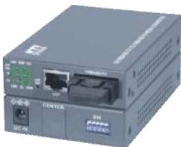
Fast Ethernet desktop media converter with 1x 10/100MBit/s 100Base-TX RJ-45 port and 1x 100Base-FX multimode / singlemode (monomode) / BiDi (WDM / SingleFiber) or CWDM port, optimized latency, auto-negotiation, auto MDI/MDI-X, dimensions 108x75.5x23mm, operating voltage +5V..+12V DC, consumption max. 2W. Operating temperature -5°C..+50°C, RH 5..95% non condensing, FCC class B, CE class B, remote port status (LED), 19" rack installation with product group 0961138 or 0961398.
