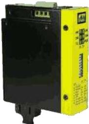
Fast Ethernet industrial fiber optic converter with 1x 10/100MBit/s 100Base-TX RJ-45 port and 1x 100Base-FX multimode, singlemode (monomode) or singlemode BiDi (WDM / SingleFiber) fiber optic port for ST / BFOC or SC connector. 35mm DIN rail mountable, fanless metal case dimensions 28x82x95mm (WxDxH), operating voltage 7V..30V DC, operating temperature -20°C..+70°C, RH 5%..95% non condensing, FCC Class A, CE/EMC Class A, EN60950 safety.
