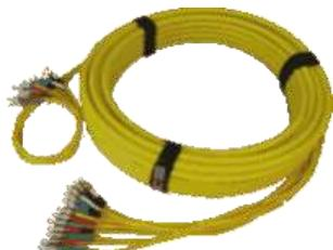
Fiber optic breakout cable (full breakout) I-V(ZN)HH. Made-to-order termination multimode OM1, OM2, OM3, OM4 or singlemode (monomode) OS2 with connectors of your choice optional on one side or on both sides with pulling- and protection element.
