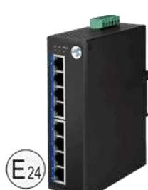
Industrial Ethernet E-Mark switch with 8x 10/100/1000MBit/s 1000Base-T RJ-45 high PoE ports (PoE+ PSE) according to IEEE 802.3at standard max. 30W /port. Input voltage 9V..55V DC redundant, power consumption max. 254W. Rugged metal case IP30, dimensions WxHxD 46x142x99mm, overload current protection, operating temperature s. Selection box, 35mm DIN rail mountable and wall mounting.
