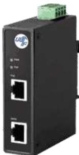
Industrial Power over Gigabit Ethernet injector, data ports 10/100/1000MBit/s 1000Base-T RJ-45, input voltage 12V..55V DC at screw terminal, output according to IEEE 802.3at standard max. 30W, consumption 1.44W + PoE. Operating temperature -40°C..+85°C, relative humidity 5%..95% non condensing, rugged metal case IP30, dimensions WxHxD 26x95x75mm, 35mm DIN rail mountable and wall mounting, overload current protection, reverse polarity protection, CE, FCC Class A
