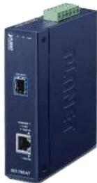
Industrial 10 Gigabit Ethernet bridging media converter with 1x 10G/5G/2.5G/1G/100MBit/s 10GBase-T RJ-45 port and 1x 10Gbit/s 10GbE SFP+ slot, 16K Jumbo frame support, input voltage 12V .. 48V DC or 24V AC redundant, alarm contact, 6kV DC ESD protection, dimensions WxDxH 32x87x135mm, operating temperature -40° .. +75°C, DIN rail mountable or wall mounting.
