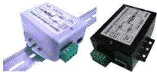
PoE Power over Gigabit Ethernet injector for direct current. Input 10..36V DC, output PoE 17W max. (48V 0,35A) according to IEEE 802.3af mode A (pins 12-36+) or mode B (pins 45+ 78-) s. Selection box, suitable for industrial use, dimensions: 85x57x36mm LxWxH, input with fuse protection, protection against short circuit, CE, UL1950, CSA 22.2, EN60950-1, FCC Class B, EN55032 Class B, operating temperature -40°C..+70°C, wall mounting, optional with DIN rail mounting kit.
