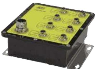
Industrial Fast Ethernet switch with 8x 10/100MBit/s 100Base-TX Fast Ethernet ports for M12 connector D coded. Operating temperature -40°C..+70°C, dimensions 163x195x60.5mm (WxDxH), protection class IP65 and IP67, operating voltage +6.5..60V DC at M23 connector, consumption: 11.5W, recessed mounting or wall mounting, inklusiver starter cable set.
