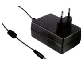
18W plug-in power supply input voltage 85V..264V AC, output voltage: s. Selection box, energy efficiency level VI, no load power consumption < 0.075W, protection against short circuit, overload, overvoltage. Plastic case, power ON LED, operating temperature -30°C ... +70°C (>50°C derating), relative humidity 20% .. 90% non condensing, dimensions LxWxH 79x54x33mm. Inner contact = +.
