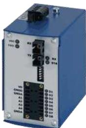
Fiber optic transmitter and receiver for up to 8x 12V - 24V DC digital switching signals / control signals via fiber optic lines (Multimode or singlemode optical fiber), operating voltage 12V..30V DC, operating temperature -40°C..+70°C. Mounting on 35mm DIN rail. Receiver: separate voltage-input for signal output with 500V DC isolation against operating voltage. Alternatively relay-output.
