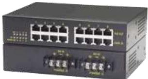
Industrial Power over Gigabit Ethernet injector with 8x 10/100/1000MBit/s 1000Base-T RJ-45 PoE ports according to IEEE 802.3at (max. 30W /port) and IEEE 802.3af standard. Fanless metal case, dimensions WxDxH 190x140x43mm, optional 19" bracket for 1 or 2 devices available. Extended temperature range, operating temperature -40°C..+70°C. Approvals CE mark Class A, FCC Class A.
