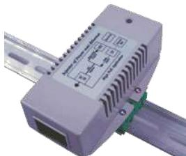
Dual Fast Ethernet (10/100 MBit/s) or Gigabit Ethernet (10/100/1000MBit/s) high PoE injector with 2x 25W PoE+ according to IEEE 802.3at and IEEE 802.3af mode B (pins 4,5+ 7,8-), plastic case, dimensions LxWxH 125x72x38mm, input voltage 100V ... 240V AC, operating temperature -25°C ... +50°C, relative humidity 5% ... 90% non condensing, FCC Class A, EN55032 Class A, EN60950-1 (2. Edition), wall mountable, optional DIN rail mountable.
