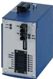
Analogue fiber optic bridge for up to 4 analogue 0..10V voltage interfaces via a fiber optic connection. Wavelength 1310nm, connector ST/BFOC, SC or E2000, dimensions WxHxD 60x100x113mm without fiber optic port and clamp terminals, operating temperature -40°C..+70°C, operating voltage 12V..30V DC. On request voltage up to 70V DC or distances up to 100km possible.
