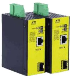
Managed Industrial Ethernet media converter with 1x 10/100/1000MBit/s 1000Base-T RJ-45 port and 1x 100/1000MBit/s 1000Base-X / 100Base-TX dual speed SFP slot for multimode or singlemode (monomode) SFP module.
